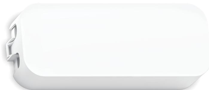
LED Driver with built-in dimmer for 12/24 V DC LED-strips with up to 75 W load. The product can be controlled wirelessly via the app or through other products from Plejd.
